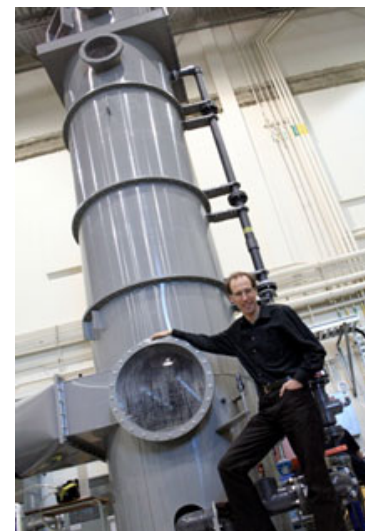
Figure 1. Professor David Keith at the University of Calgary, standing next to the tower of a prototype carbon sequestration machine, capable of capturing about 1 tonne of CO 2 per day.
